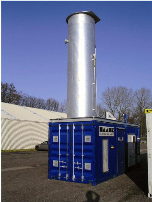
**Picture 1: Mobile high-temperature flare** for the disposal of explosive mixtures from tank farms. The total combustion capacity amounts to 5MW with a suction capacity from 500 to 3,000m<sup>3</sup>/h
